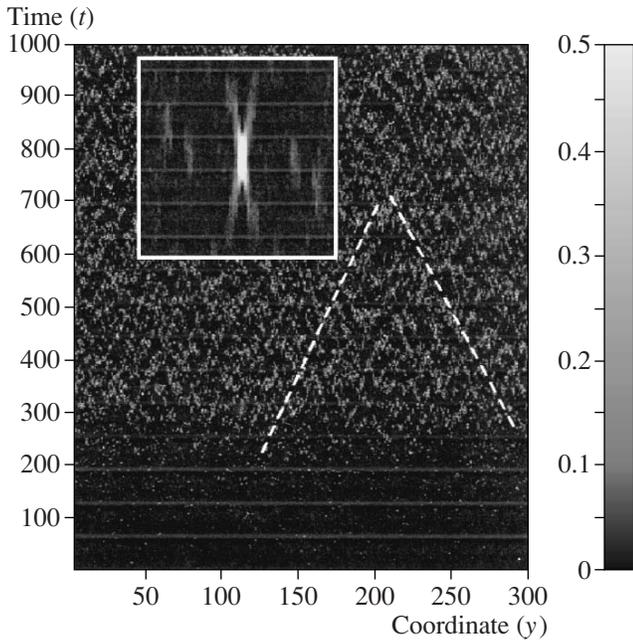
**Fig. 1.** Spatiotemporal map of jump distribution represented by the  $M(t, y)$  matrix, with the intensities indicated by gray tint scale on the right. The initial stage corresponds to establishment of a stationary process. Dashed lines correspond to the characteristic velocities of wave propagation (pre- and aftershocks). The inset shows the corresponding  $G(t, y)$  correlation function.
